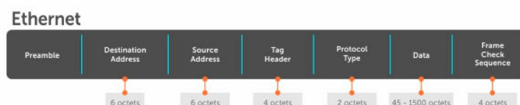
Figure 130. Tagged Frame Format
